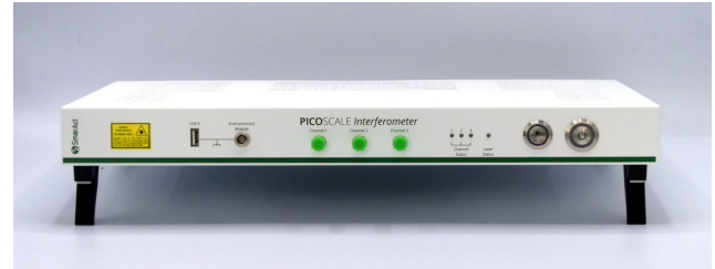
Figure 2. The PICO-SCALE Interferometer V2. Up to three sensor heads can be connected to the controller, which contains a laser source, detection electronics, FPGA-based fast data processing and several interfaces.
