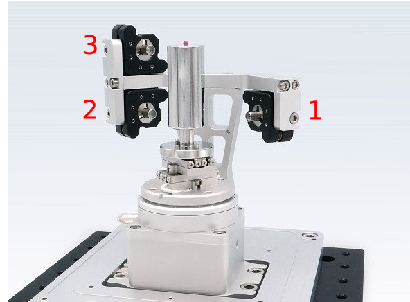
Figure 2. Experimental setup. Three PICOSCALE sensor heads with line focused probe beam are targeting a polished cylinder, which is mounted on an xy- and a rotary stage. See text for details.
