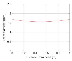
Figure 2. Beam diameter as function of working distance.
