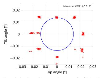
**Figure 3.** Angular working range for a sensor head C03 and a target mirror at a distance of 50 mm. The typical minimum angular working range was determined to  $\pm 0.013$  degrees.
