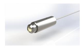
The C03 is a sensor head type optimized for moderate working distances and using retro-reflectors as target. The probe beam is enlarged so that its divergence is reduced and more optical power can be collected after reflection at the target mirror.
