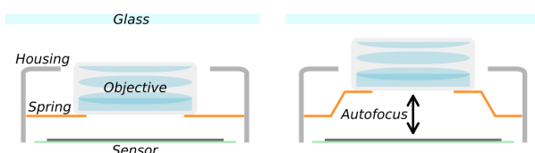
Figure 1. Schematic representation of a smartphone camera unit. The optics sit in a flexible mount which can be moved to allow for focusing.
