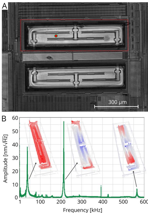
**Figure 2. Modal analysis of the motion sensor through a silicon window.** A) The vibrations were first measured at the indicated point. B) The amplitude spectral density plot shows multiple resonance peaks. At the indicated peaks a modal analysis was performed of the part of the structure that is indicated by the red box in A). The inset figures show a 3D rendering of the motion of the structure.
