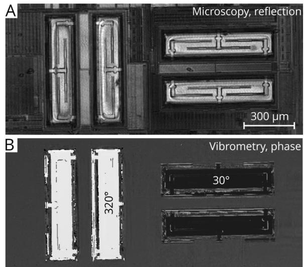
**Figure 3. Relative motion of multiple objects.** A) Confocal microscopy image showing a total of 4 mobile structures. B) The motion sensor was actuated at 37.4 kHz and the phase image shows the phase with respect to the shaker stage signal. The phase is gray-scale coded ( $0^\circ$  is black,  $359^\circ$  is white), the difference in phase between the mobile structures is  $\approx 70^\circ$ .
