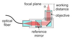
**Figure 1.** Schematic drawing of the F03 sensor head. The light from the optical fiber is collimated and split into a reference and measurement beam. The measurement beam is turned by 90° and focused on the sample by the objective lens.
