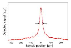
**Figure 3.** Measuring the working range of an F03 sensor head with 0.25 NA objective. The reflected signal was recorded while moving the sample (a mirror) up and down. The signal, routed through the single mode optical fiber, was measured by the photo diode inside a **PICO**SCALE Vibrometer controller. Due to the confocal arrangement of the optical path, the recorded intensity peak is very sharp, resulting in a small working range. In this case, the full width at half maximum is 35 µm.
