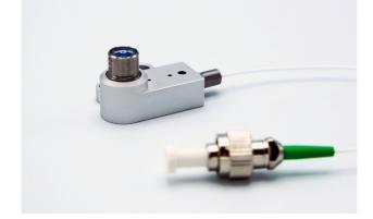
The F03 sensor head is intended for use with the **PICO**SCALE *Vibrometer* or the **PICO**SCALE *Interferometer*. The sensor head contains a Michelson interferometer and can be combined with various objectives to focus the measurement laser beam into a micrometer sized spot. This allows to measure displacements of microscopic targets at pm resolution. In combination with the **PICO**SCALE *Vibrometer*, the sensor head can also be used for high-resolution confocal microscopy.
