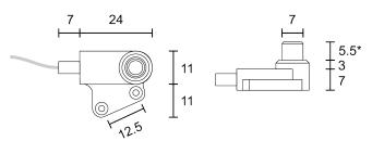
*Figure 6.* Schematic drawing of the F03 sensor head with objective, the dimensions are in mm.
