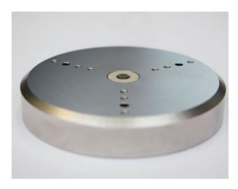
The shaker stage is intended for use with the PICO-SCALE *Vibrometer*. It allows the mechanical excitation of samples at frequencies of up to 1.5 MHz. Applications include the excitation of motion sensors and micro-cantilevers in order to find their resonance frequencies and bending modes. The shaker stage can also be used as a stable passive mount for small samples.
