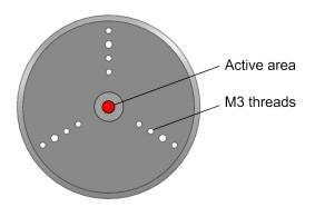
**Figure 1.** Schematic drawing of the shaker stage. Vibrations are induced at the active area (shown in red).
