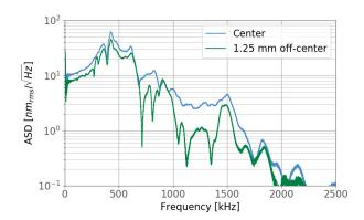
**Figure 2.** Typical response of the shaker stage measured with the PICOSCALE Vibrometer. The 5  $V_{PP}$  drive signal was generated by the stage controller, no sample was mounted. At the vertical axis the actual amplitude spectral density is shown at each frequency. The blue curve was recorded at the center of the active area, up to 1.6 MHz the induced amplitude is more than 1 nm<sub>rms</sub>/ $\sqrt{\text{Hz}}$ . The green curve was recorded 1.25 mm towards the periphery.
