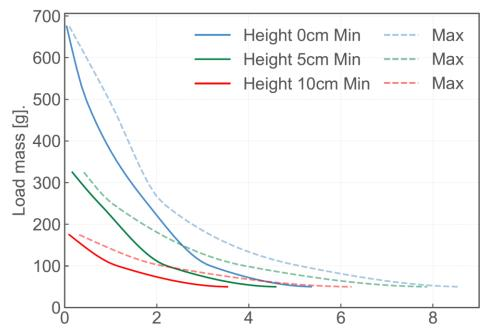
Radial horizontal displacement of load (center of mass) from the positioning systems mechanical interface center [cm].
