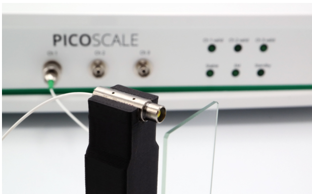
Figure 1. Experimental setup. A PICOSCALE focusing sensor head is directed on a microscope slide and tracks its vibrations.
