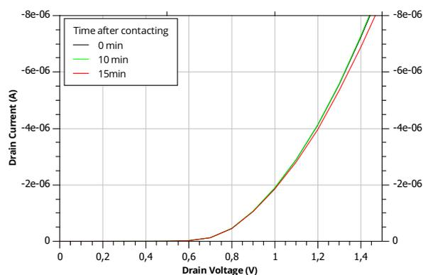
**Figure 2.** **a)** Image of the **SMARPROBE** graphical user interface. Key feature are *point&click* and *image-on-move*. **b)** Four nanoscopic tips contacting a transistor of a 14 nm technology node processor. **c)** I-V curve of the transistors drain contact measured against ground. The electrical contact between tip and drain contact is stable for around 15 minutes.
