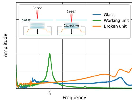
**Figure 2.** Mechanical response of a smartphone camera unit. An intact camera shows a clear peak at  $f_c$ , green curve, as compared to the protective cover glass and a damaged camera unit, blue and orange curves respectively. Inset: Measurement principle showing how the confocal optics of the PICO SCALE Vibrometer allow to measure on selected surfaces.
