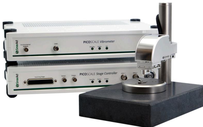
**Figure 1.** The **PICOSCALE Vibrometer** consists of a controller, a three-axis positioner that holds the microscope objective, a shaker stage to mechanically actuate the sample and software to control the measurements and to analyze the results.
