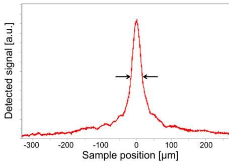
**Figure 3.** Measuring the working range of an F03 sensor head with 0.25 NA objective. The reflected signal was recorded while moving the sample (a mirror) up and down. The signal, routed through the single mode optical fiber, was measured by the photo diode inside a PICOSCALE Vibrometer controller. Due to the confocal arrangement of the optical path, the recorded intensity peak is very sharp, resulting in a small working range. In this case, the full width at half maximum is 35 µm.
