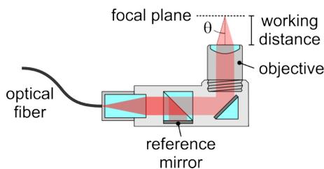
**Figure 1.** Schematic drawing of the F03 sensor head. The light from the optical fiber is collimated and split into a reference and measurement beam. The measurement beam is turned by 90° and focused on the sample by the objective lens.
