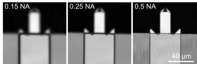
**Figure 5.** Micro-cantilever imaged with the different objectives. In all images, recorded at 10 kilopixel and unprocessed, the  $16 \mu\text{m}$  wide cantilever can be distinguished. The 0.5 NA objective provides the image with the highest resolution.
