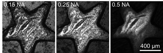
**Figure 4.** Feature on a coin imaged with the different objectives. All images were recorded at 1 Megapixel and are unprocessed. Due to its larger working range, the 0.15 NA objective provides the image in which the  $\approx 0.2 \text{ mm}$  high structure can be best appreciated. In the images recorded with the objectives with a higher NA, the background remains dark and it becomes more difficult to recognize the structure.
