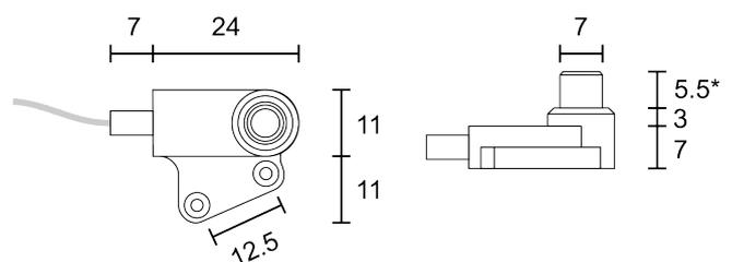
**Figure 6.** Schematic drawing of the F03 sensor head with objective, the dimensions are in mm.
