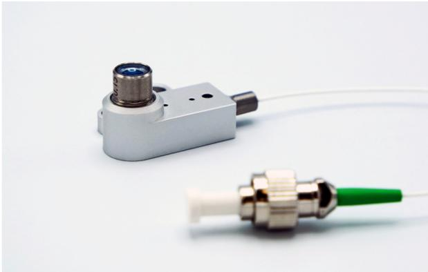
The F03 sensor head is intended for use with the **PICOSCALE Vibrometer** or the **PICOSCALE Interferometer**. The sensor head contains a Michelson interferometer and can be combined with various objectives to focus the measurement laser beam into a micrometer sized spot. This allows to measure displacements of microscopic targets at pm resolution. In combination with the **PICOSCALE Vibrometer**, the sensor head can also be used for high-resolution confocal microscopy.
