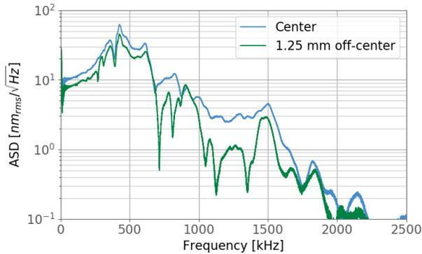
**Figure 2.** Typical response of the shaker stage measured with the PICOSCALE Vibrometer. The  $5V_{pp}$  drive signal was generated by the stage controller, no sample was mounted. At the vertical axis the actual amplitude spectral density is shown at each frequency. The blue curve was recorded at the center of the active area, up to 1.6 MHz the induced amplitude is more than  $1\text{ nm}_{rms}/\sqrt{\text{Hz}}$ . The green curve was recorded 1.25 mm towards the periphery.
