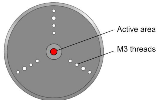
**Figure 1.** Schematic drawing of the shaker stage. Vibrations are induced at the active area (shown in red).
