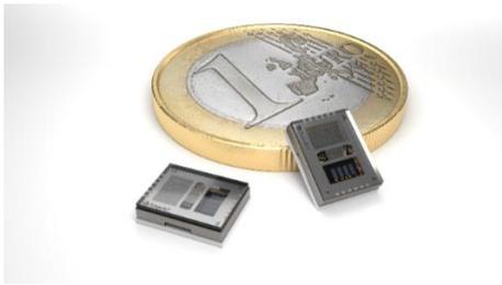
The **METIRIO** Readhead is an analog high precision encoder, designed and manufactured to meet the most stringent market requirements for closed-loop nano-positioning. The readhead constitutes the core of the METIRIO encoder, and is encapsulated in a small package, featuring maximum miniaturization, low noise and high bandwidth. It is suited for the deployment in UHV and in conjunction with linear, rotary and convex scales.
