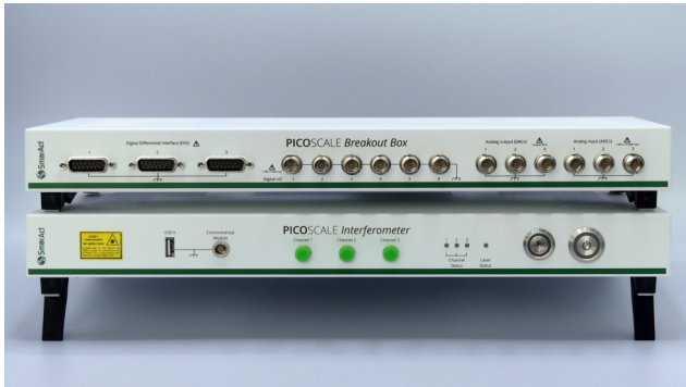
Figure 1. Photograph of the PICOSCALE Interferometer V2 with the Breakout Box on top.
