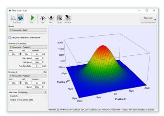
The Precision Tool Commander uses driver plugins to communicate with third party devices. Data measured by these external sensors can be correlated by the PTC to the position data of the stages. Thus, allowing to perform 1D and 2D position scans while logging additional sensor data. The PTC is able to display these 3D data sets as well as export them as an image or a CSV file. Please feel free to contact our application scientists to
