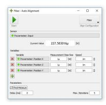
The Align software module makes also use of the Precision Tool Commanders ability to communicate with third party measurement equipment. It uses an iterative algorithm to find the optimum position for defined axes of a positioning system to minimize or maximize an input value measured by the selected sensor. Typical Applications for the Align Module of the PTC are fiber coupling, beam-profiling, quality assurance and assistance for micro-assemblies.
