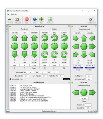
The dashboard represents an easy and intuitive way to control SmarAct stages independent of their complexity from single stages to our hexapod-like SMARPODs and TRIPODs. Stages can be moved by direct input of the destination position, or by using your computers mouse. Also multiple positioning simultaneously systems can be controlled with the PTC, giving you access to a high number of stages from a single software.
