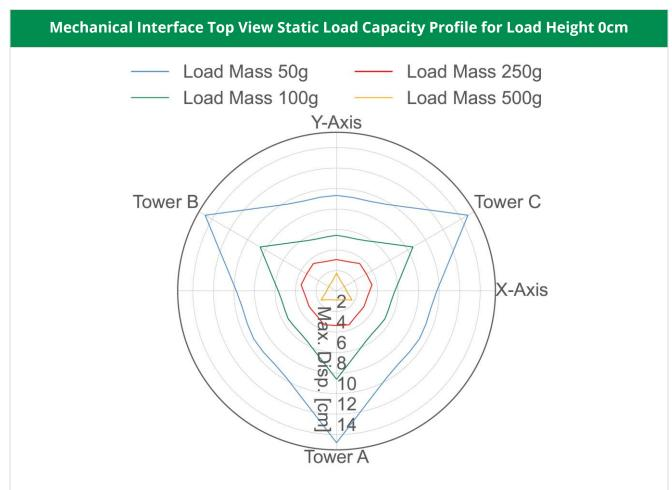
With increasing load the possible load mounting area (area inside the respective colored line) becomes smaller. The highest load is supported only close to the center of the mechanical interface of the motion system.
